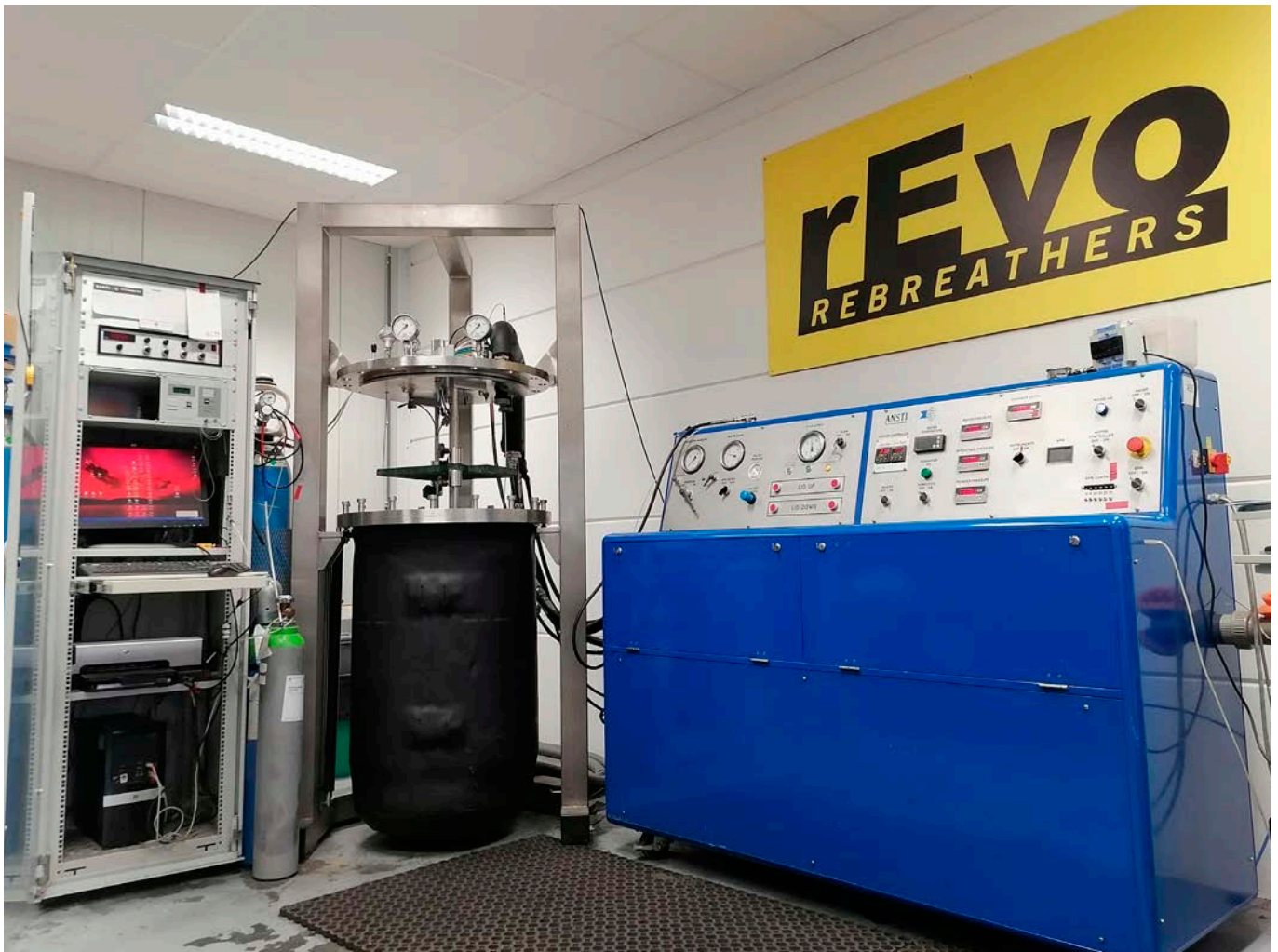
ABOVE: Breathing can be simulated on the Ansti machine and all kinds of R&D tests can be performed. TOP RIGHT: Devices ready to be delivered to future rebreather divers. BOTTOM RIGHT: BOV 6 – The rEvo BOV (Bail Out Valve).
